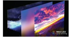
Mini LED backlighting improves control of lighting and contrast ratio. The small size of the mini LEDs forming the backlight allows for the creation of 2304 individually controlled zones delivering deeper blacks and brighter whites. Rich HDR content can now be viewed as it was intended with unmatched contrast and precise reproduction.
