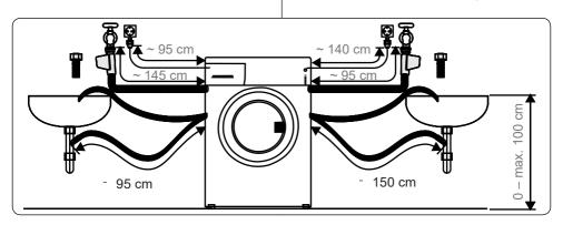
must only be connected to your water supply using the supplied new fill hose. Old hoses must not be reused.
