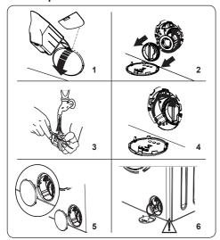
The pump filter system in your Washing Machine prolongs the life of the pump by preventing lint from entering your machine. We recommend that you clean the pump filter every 2 months.
