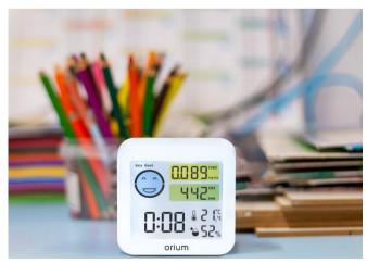
When using batteries: VOC and CO2 measurements are not performed automatically to save batteries. Perform the measurements manually as described. The new VOC and CO2 measurements are displayed at the end of the 5-minute countdown. Then the Quaelis meter is again in standby mode (no VOC and CO2 measurements).
