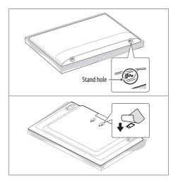
Screw length from outer surface of back cover should be under 8 mm. (Only 24/28LT66\*)
