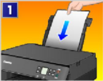
1. Load paper into the rear tray correctly.
