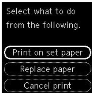
Use the ▲ ▼ buttons to select the appropriate action, then press the printer's **OK** button.
