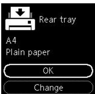
If the page size on the LCD matches the size of the paper loaded in the rear tray, select **OK**.
