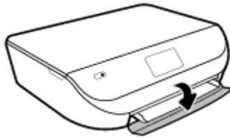
2. Pull the paper tray out and slide the paper-width guides outward.
