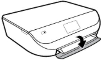
2. Pull out the paper tray, slide the paper-width guides outward, and then remove any previously loaded media.
