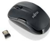
The Wireless Mouse W1200 uses the latest wireless 2.4 GHz technology, and a high-resolution 1000 dpi optical sensor to give you the precision and reliability you need. Sporting a compact design with a stylish black finish, the W1200 wireless mouse is well suited to all environments and to each user whether right or left handed.
