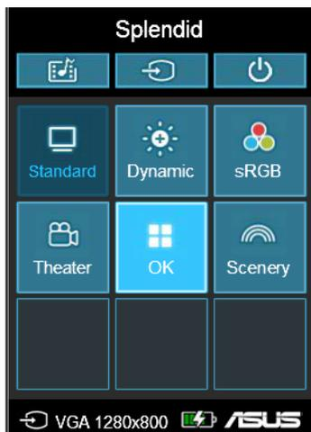
Press this button while on battery mode to activate different brightness modes. The time (HH:MM) under the icon shows the estimated battery life in that brightness mode.
