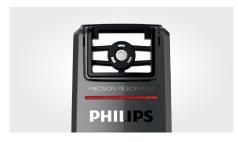
The free-floating microphone is decoupled from the device's housing, which guarantees that almost no background, touch, click, air or structure-borne noise is recorded. This technique is derived from studio microphones to make sure there are no sound distortions whatsoever and to guarantee outstanding speech recognition results.
