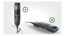
Being on the cutting edge of technology, the SpeechMike Premium Touch comes with an integrated motion sensor, making it the first stationary dictation device that can be controlled by the movement of your hand. It detects when it's put on the table, mutes the microphone, and once it is being picked up again it unmutes the microphone. In addition to that, custom events can be programmed, e.g., to pause and to continue the recording.
