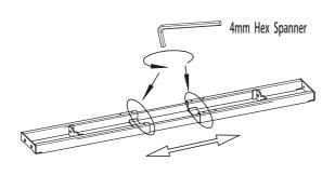
Attach legs to the beam using 8 of M6\*12 screws.
