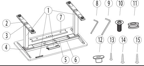
1 Loosen the M6\*10 screw on the beam with 4mm hexagon wrench, then adjust the lengt of the beam according to the tops, and finally fix the beam with the M6\*10 screw in the screw package and the screw on the beam.
