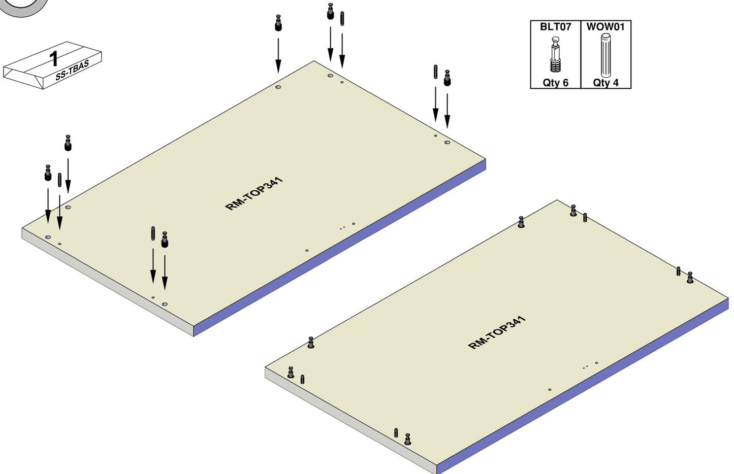
Prepare all the panels by inserting the listed fittings into the corresponding holes.
