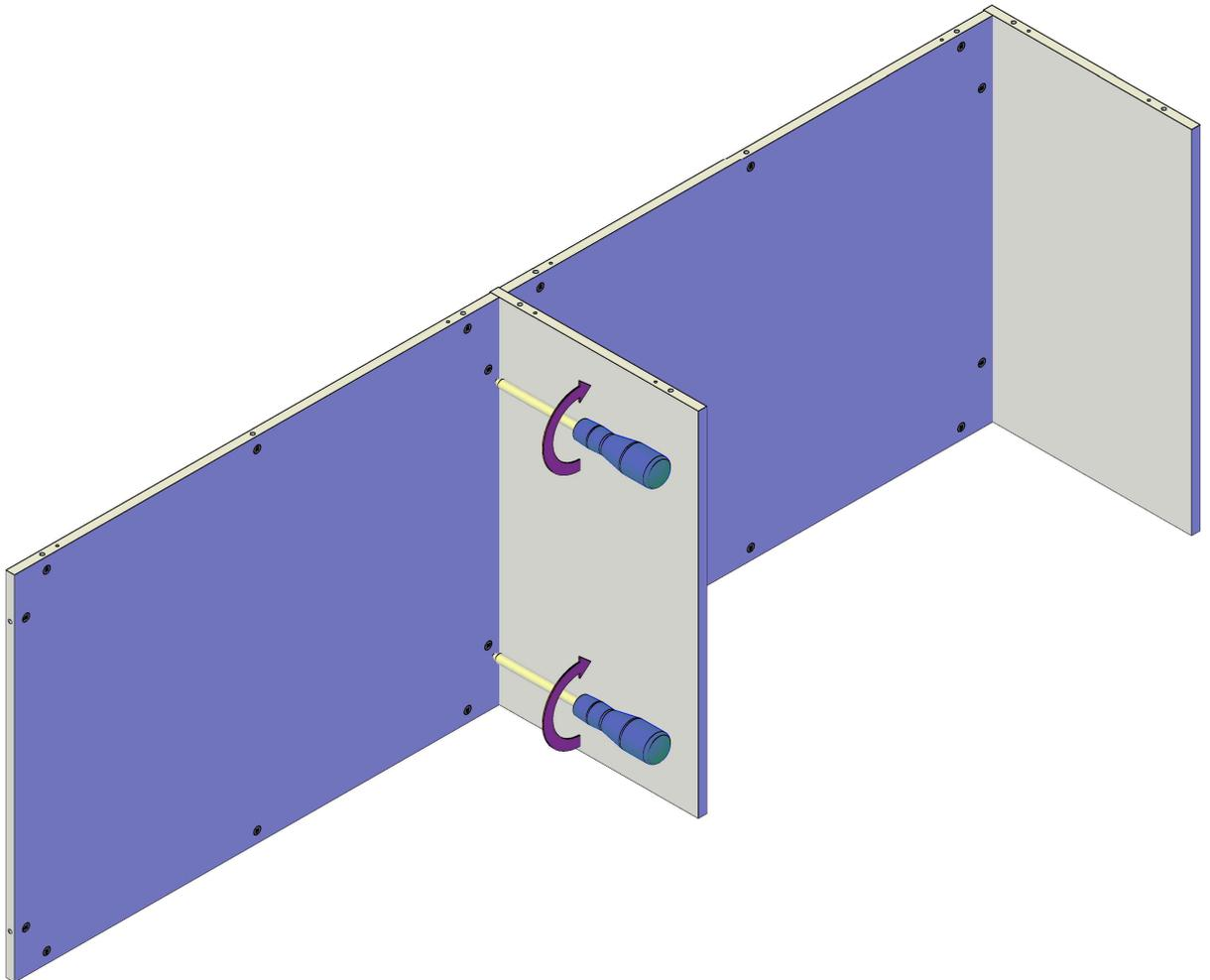
Join the panels together and tighten all cam fittings
