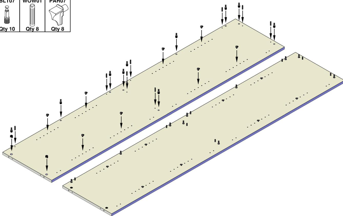
Join the panels together and tighten all cam fittings
