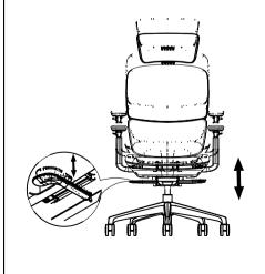
4. Tilt lock/seat depth adjustment
