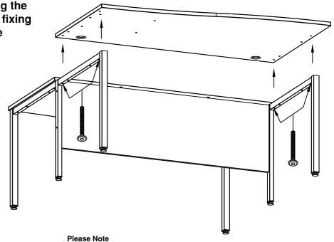
Fixing point B is only to be used if the desk top is old style ( pre 2020 ) and there is no drilled hole for the rear fixing insert.
