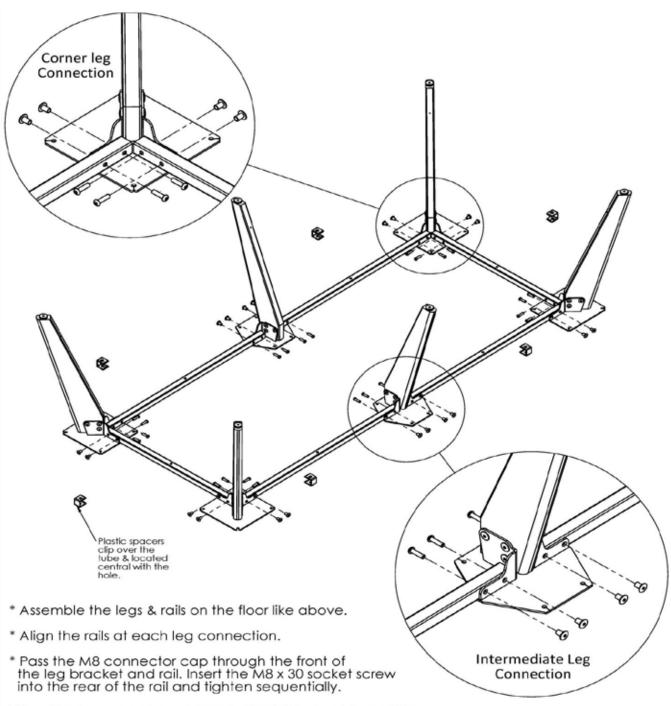
\* Turn the frame work over, locate the table top into position and secure in place with M6 x 15 connector bolts through the leg brackets and M6 x 50 connector bolts through the rails.
