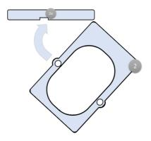
!Attention! Make sure that the metal rail is inside the recess on the underside (2a) of the slide (2).
