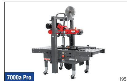
3M-Matic™ Adjustable Case Sealer 7000a Pro is an adjustable top and bottom belt drive to dependably seal uniform cases at up to 40 cases per minute.
