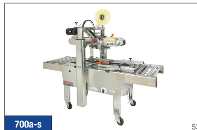
3M-Matic™ Adjustable Case Sealer 700a-s stainless steel has advanced features to seal uniform cases up to 30 per minute. Dual masts with dual lead screws for stability and uniform height adjustments. Adjustable top and bottom belt drive system for reliable conveyance of heavier or tall/light boxes. Compression rollers position each box for precise tape sealing. Stainless construction for corrosive environments.
